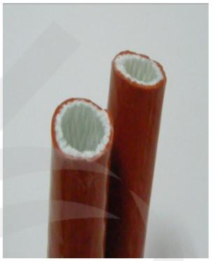
500°F (260°C); up to 2000°F (1090°C) for 15-20 minutes; and up to 3000°F (1650°C) for 15-30 seconds. When exposed to flames, the silicone rubber transforms into a crust, creating a protective SiO2 refractory layer. Fire Sleeving is constructed from high bulk glass fibre brad sleeving. Excellent modulus of elasticity makes it an ideal choice for bundling hoses, tubes and cables in a variety of hostile environments.
