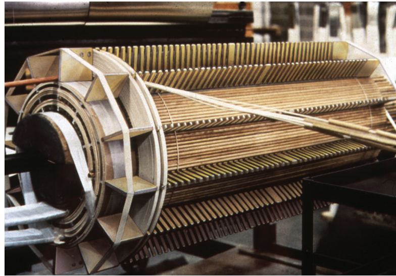
Ventilated Dry-Type Transformer Coil. Both SG-200 and FHT Laminates are used in a wide variety of dry-type transformer
