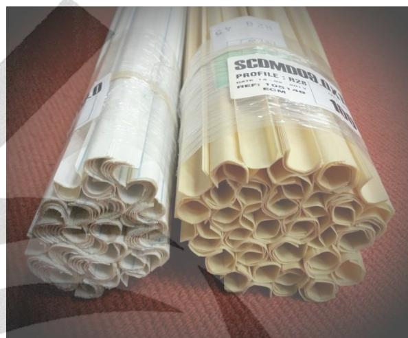
Slot Closures come in a full range of shapes and can be used on any type of standard motor (stators and Rotors). Shapes are supplied in batches of 100 units 700mm long. Each shape can be cut without risk into submultiples of 700 mm using hand or mechanical shears.
